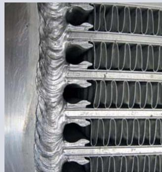
Cool-Line uses patented AKG hollow profiles to reduce local peak strains. This way the strength of heat exchangers is significantly increased and their service life time considerably prolonged.
